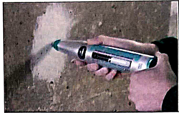
Rebound Hammer Test
